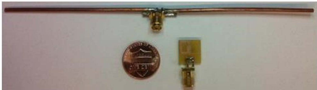
Figure 158. Size of ESA compared to half-wave dipole and a penny.
