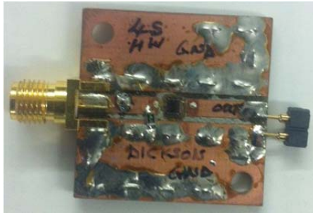
Figure 107. Rectifier circuit 50 \Omega Test fixture.
