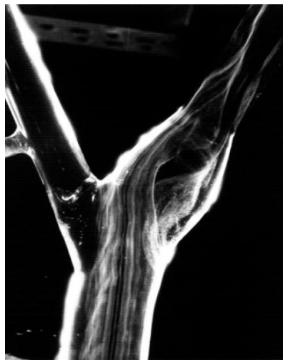
Figure 4: Visualization of flow in a glass model of carotid bifurcation[15].
