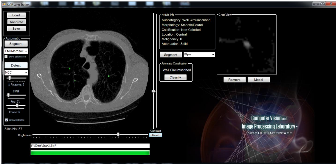
Figure 37: Screenshot of the designed interface. The interface is meant to be simple, fast and functional. Most of the interface consists of the slice view (Axial slice shown above), while the regions surrounding the slice view hold toolboxes which assist the user in annotating nodules. Note: the annotation shown in the right-hand pane of the interface is just for demonstration purposes and does not pertain to a real nodule.
