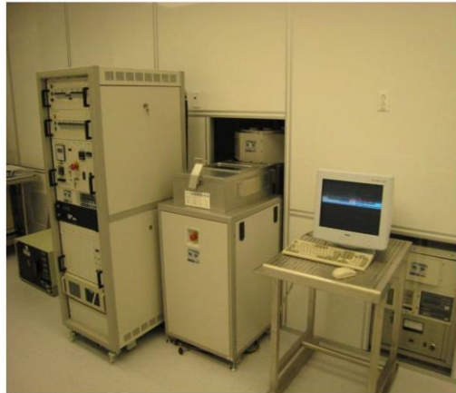
Fig. 23. DRIE tool at the MNTC's cleanroom.
