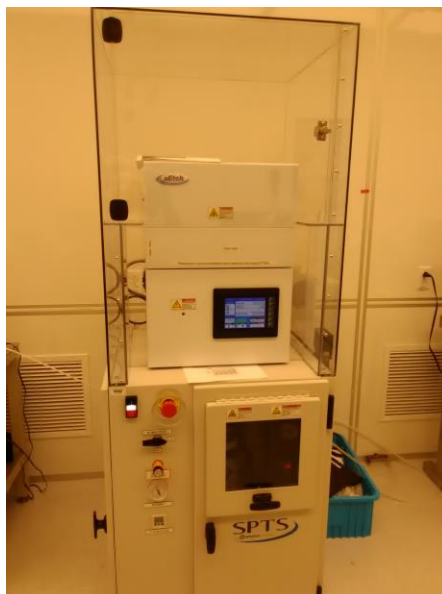
Fig. 27. Anhydrous HF etch tool in the cleanroom.
