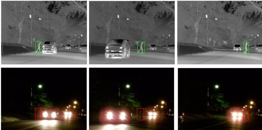
Figure 6.1. An illustrative example of night problems. The upper sequence shows a pedestrian crossing the street using thermal images. The lower sequence shows the same scene using visible images where the pedestrian is very difficult to detect because of both the glare from the headlights of oncoming traffic and the low light of the night scene.
