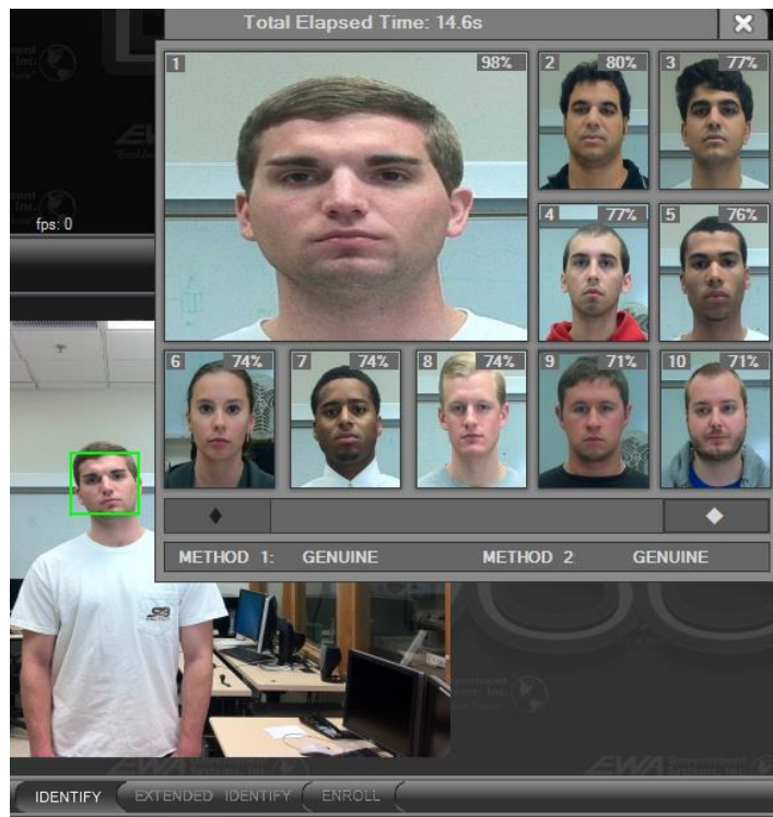
FIGURE 39 – True Positive Identification; Confidence Level = 98% Distance = 5 feet, Illumination ON, Roll = +15°
