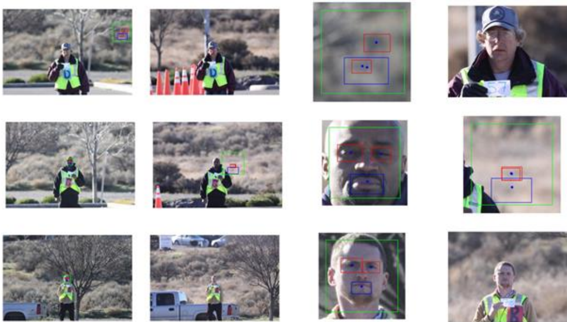
FIGURE 28 - Face detection errors at 80 and 100 and 150 meters
