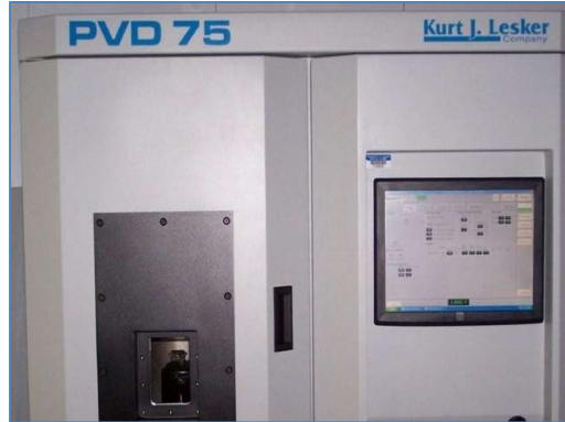
Figure 4.13. PVD 75 RF/DC sputtering system from Kurt J. Lesker. Both 3” and 4” targets can be used in the system and it is capable of co-sputtering.
