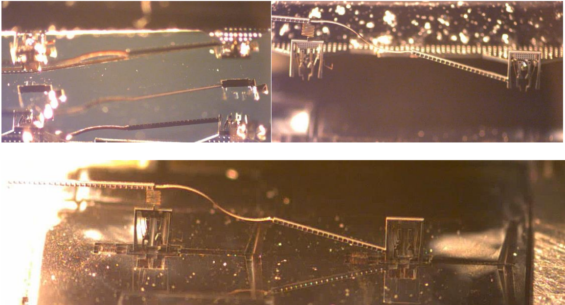
Figure 4.27. Picking-up, rotating, and placing for sAFAM assembly
