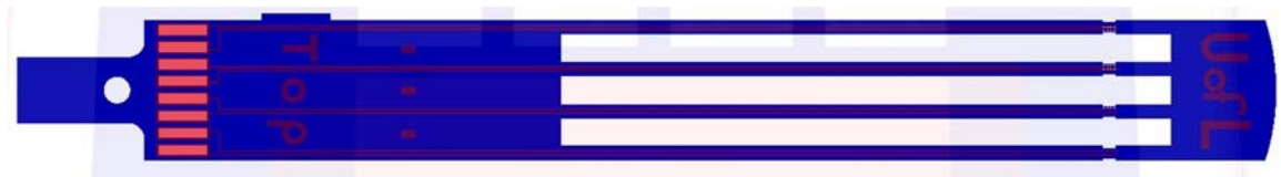
Figure 2.3: P-MEA device, version 2. Thin-film metal conductor sandwiched between two layers of insulating polymer material.
