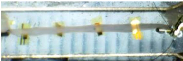
Figure 5.8: A P-MEA embedded ECT under force measurement. The remnants of the P-MEA can be seen in the still-embedded pads in the ECT. The left hook is attached to a force transducer and the right anchor is movable to stretch the ECT.
