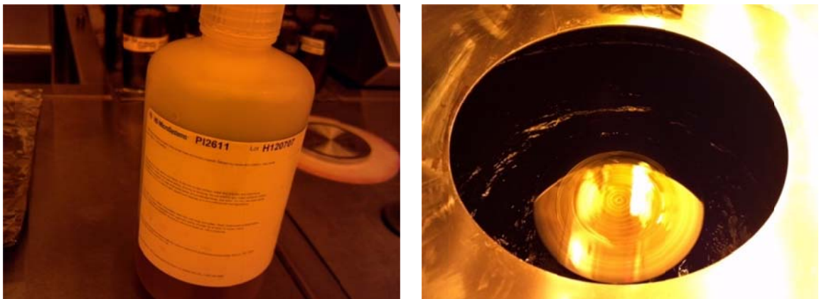
Figure 3.2: (a) PI2611 bottle stored in refrigerator. (b) Spin-coating PI-2611 on a silicon wafer.
