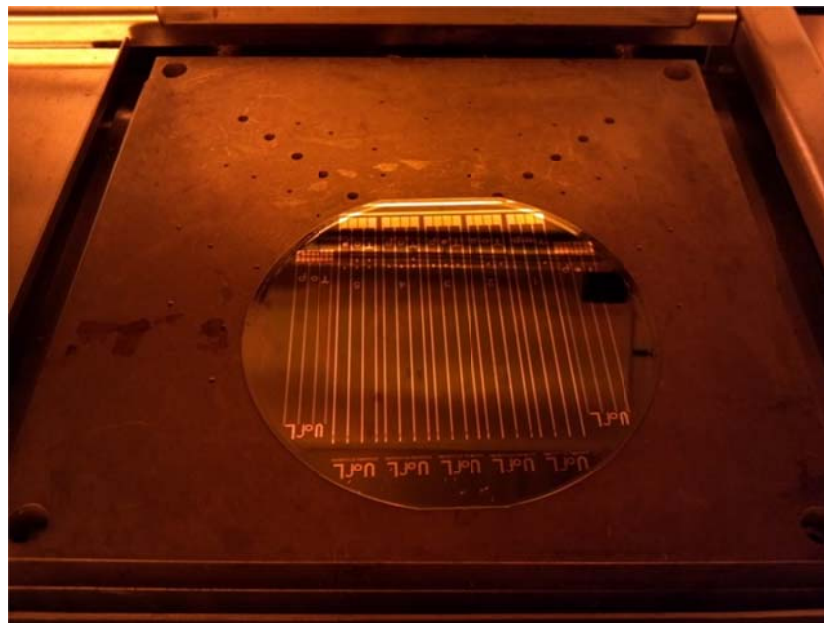
Figure 3.11: Second layer of polyimide – soft bake on hotplate prior to vacuum curing.
