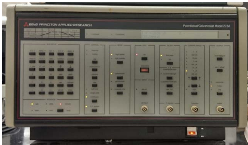
Figure 4.5: Model 273A, Potentiostat/Galvanostat (Princeton Applied Research, Oak Ridge, TN); used for the EIS experiments and measurements.
