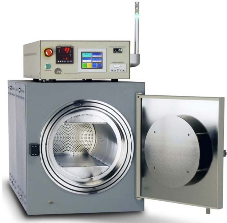
Figure 3.3: PI cure vacuum oven from Yield Engineering Systems. Wafers (up to 6” in diameter) are loaded vertically and nitrogen gas flows in a perpendicular direction (to the chamber), across the surface of the wafer. (Image source: company website).
