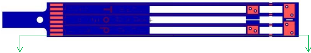
Figure 3.1 (a): P-MEA device. Green arrow lines show the approximate location of the cross-sectioning. The device design used for the example is version 3.
