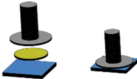
Figure 41: Flow Visualization Device: A membrane polarized between a wire and an optically-transparent conductive indium tin oxide coated slide is inspected in an inverted optical microscope during operation.
