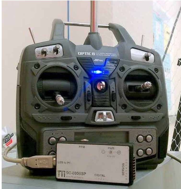
FIGURE 2.9: SC-8000SP (front) Connects RC Transmitter (back) to Controller Client PC
