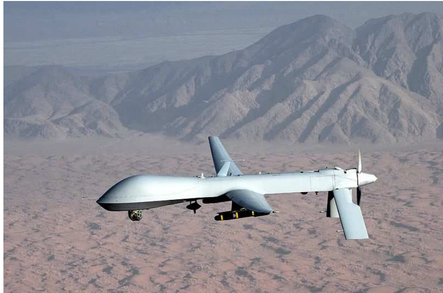
FIGURE 1.7: The Predator RQ-1L UAV (General Atomics) is capable of staying for as much as 40 hours in the air.
