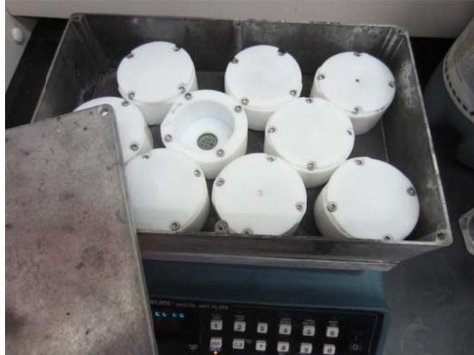
Figure 47. Nine etch cells are shown on the hot plate in the aluminum enclosure with the lid off to the side. One etch cell is shown with the PTFE lid removed, showing the silicon die and its 9 respective etch cavities.
