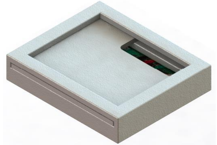
Figure 3.47: Top and bottom 3D rendering of housing
