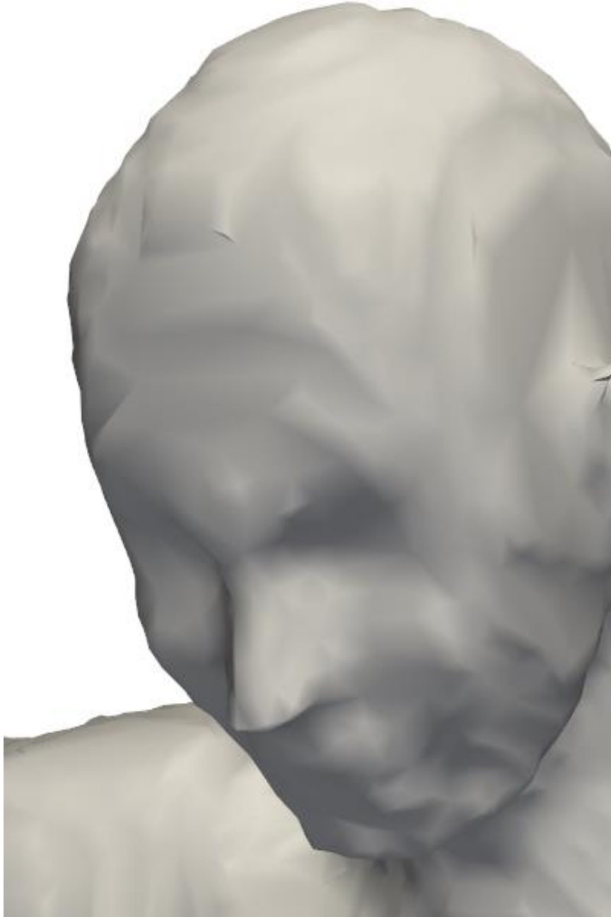
FIGURE 15 - Surface obtained by smoothing the surface generated by the marching cubes algorithm
