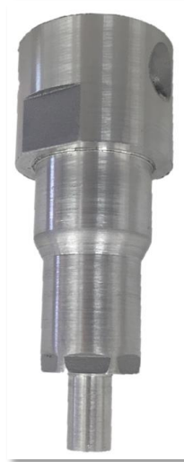
Figure D.8. Fuel injector re-designed, simulated and 3D printed by students
