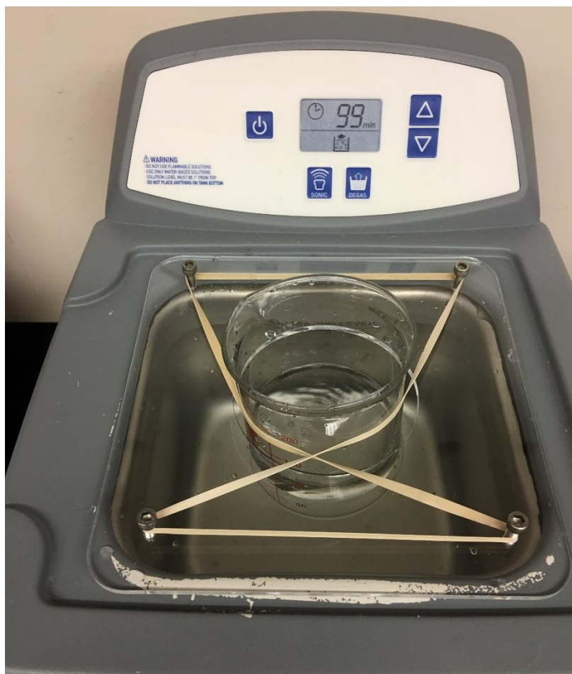
Figure 3. 19 PDMS Substrate in an Ultrasonic Acetone Bath
