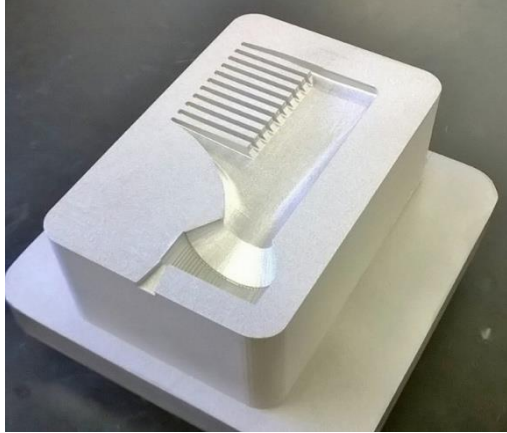
Figure 6.6 Injection mold with conformal cooling channels fabricated by L-PBF using 420 stainless steel powder ( D_{50} : 12\ \mu\text{m} ) at a layer thickness of 10\ \mu\text{m} .
