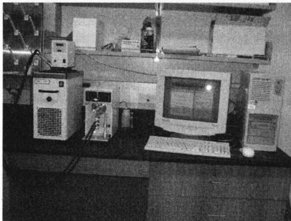
Figure 21. Complete experimental setup showing the circulator, viscoelastic analyzer and control computer.
