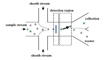
Figure I-7 Hydrodynamic focusing for detection (Wang et al. (2005)).
