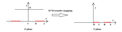
Figure III-12 The coplanar electrodes distribution and SCM transfer mapping (Sun et al.(2007)).
