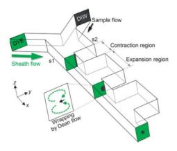
Figure I-11 3D hydrodynamic focusing with one sheath stream (Lee et al. (2009)).
