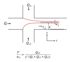
Figure I-13 The asymmetric hydrodynamic focusing (Lee (2006)).
