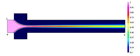
Figure 0-1 Sample flow concentration due to hydrodynamic focusing.
