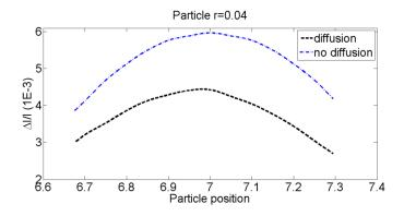
Figure V-3 Comparison of current sensitivity due to the presence of a lowconductivity particle with and without molecular diffusivity.
