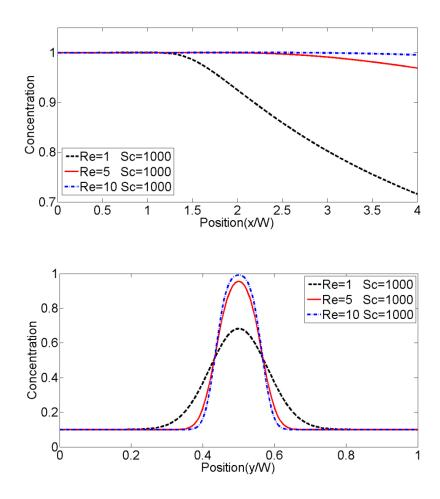
Figure 0-4 The concentration profiles at different Reynolds numbers by fixing Schmidt number.
