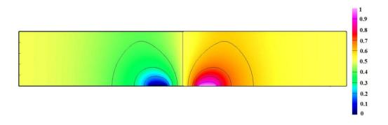
Figure III-15 Potential distribution in a 2D channel.
