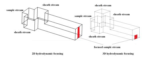
Figure I-8 Two types of hydrodynamic focusing.
