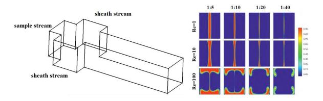
Figure I-14 Distribution of the focused sample stream for three different Reynolds number and four different focusing ratios (Blonski et al. (2011)).
