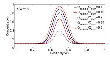
Figure 0-7 Concentration profiles for varied relative flow rate.
