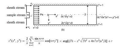
Figure I-12 The concentration distribution function (Wu (2005)).
