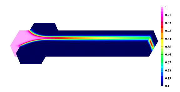
Figure 0-10 Ion concentration distribution for hydrodynamic focusing.
