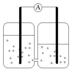
Figure I-4 Basic schematic of a traditional Coulter Counter.
