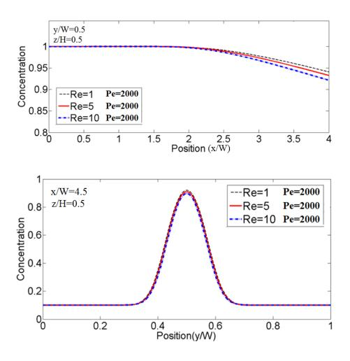
Figure 0-14 The concentration profiles at different Reynolds numbers by fixing the Peclet number.
