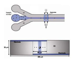
Figure I-18 A microfluidic Coulter Counter by choosing oil as the sheath stream (Bernabini et al., 2011).
