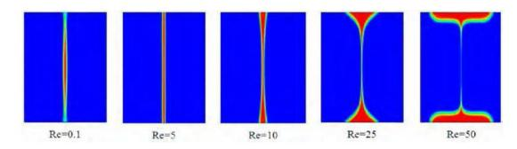
Figure I-15 Focused sample stream width considering the Reynolds number variation Blonski et al. (2011).
