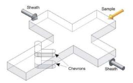
Figure I-10 Chevron-based sheath flow design. (Howell et al. (2008)).
