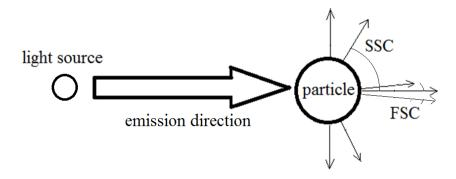
Figure I-2 Schematic representation light scattering (eventsHerzenberg et al. (2002)).
