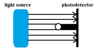
Figure I-3 Light-blocking technique (Zhang et al. (2009)).
