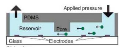
Figure I-1 Microfluidic particle detection chip (Saleh and Sohn (2002)).
