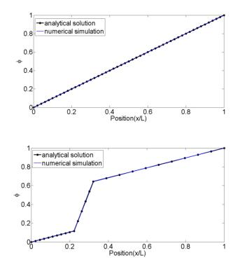
Figure III-11 Comparison of electric potential distribution along a bar with different conductivities. Top one is the case with uniform conductivity, bottom one is the case with non-uniform conductivity.
