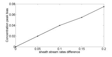
Figure 0-22 Correlation between the concentration peak bias and sheath stream flow rates difference.
