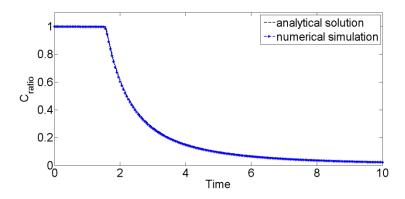
Figure III-9 Comparison with the analytical and numerical solution for the convection only situation.
