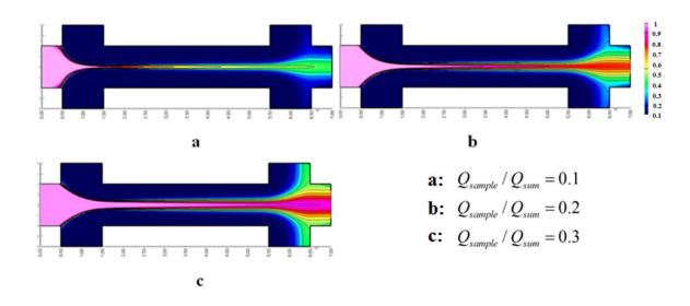
Figure 0-33 Concentration contours with different sample stream flow rates.
