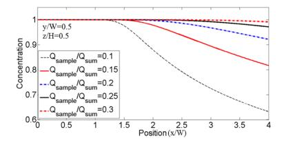
Figure 0-18 Concentration along the center line for varied relative flow rates.
