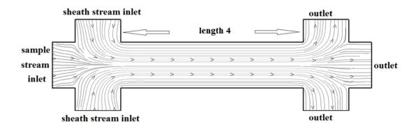
Figure 0-32 The streamlines in a three-inlet/three-outlet micro-channel device.
