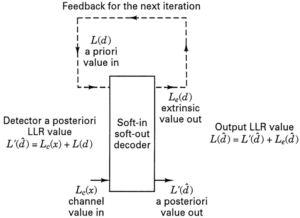
**Figure (13)** : soft input/soft output decoder (for a systematic code).
