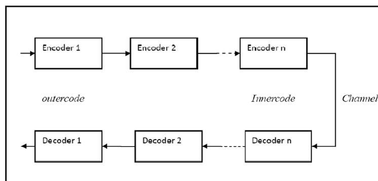
**Figure (10):** Principle of Concatenated codes
