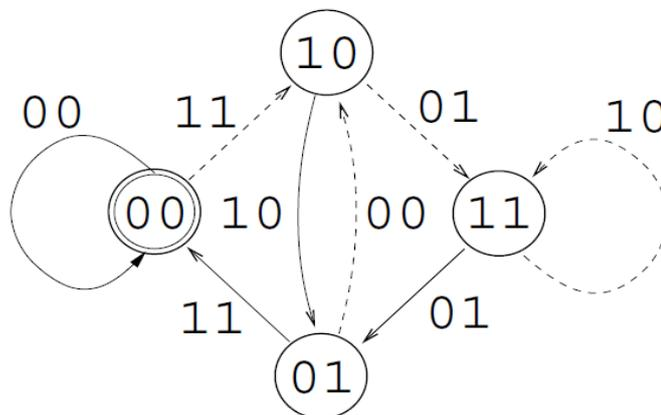
**Figure (23)** : A state machine code with a rate-1/2. The bit pairs on the transition edges represent encoded output bits.
