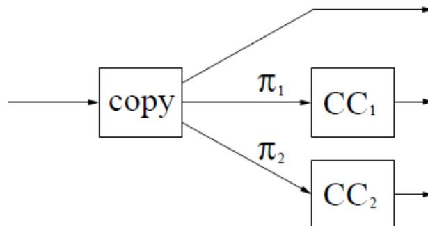
**Figure (26):** A circuit diagram for a classic rate-1/3 Turbo code. The "copy" FSM simply copies the input to the three outputs. The two component codes CC1 and CC2 are convolutional codes.
