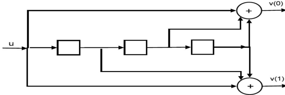
**Figure (5) :** A binary nonsystematic feedforward convolutional encoder
