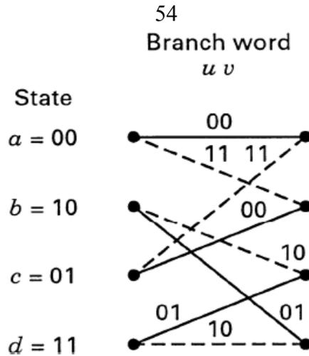
**Figure 17(b):** Trellis structure for the RSC code in Figure 17(a).
