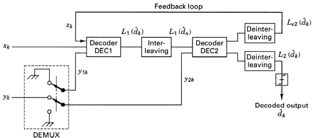
**Figure (19):** Feedback decoder.
