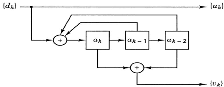
**Figure 17(a)** :Recursive systematic convolutional (RSC) code.
