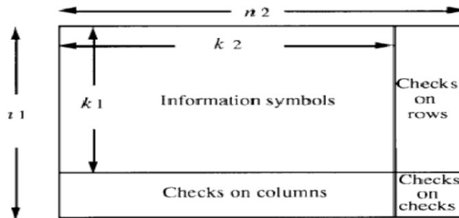
**Figure (11):** Construction of product code  $P = c^1 \otimes c^2$
