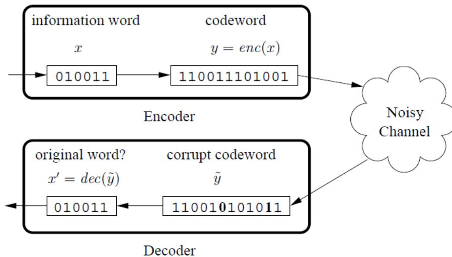
**Figure (1):** The high-level model of an error-correcting code. An information word  $x$  of length  $k$  is encoded into a longer code word  $y = enc(x)$  of length  $n > k$ . This code word  $y$  is sent over a noisy channel, and a corrupt word  $\tilde{y}$  is received at the other end. This corrupt word is then decoded to a word  $x' = dec(\tilde{y})$ , which hopefully is equal to the original information  $x$ .
