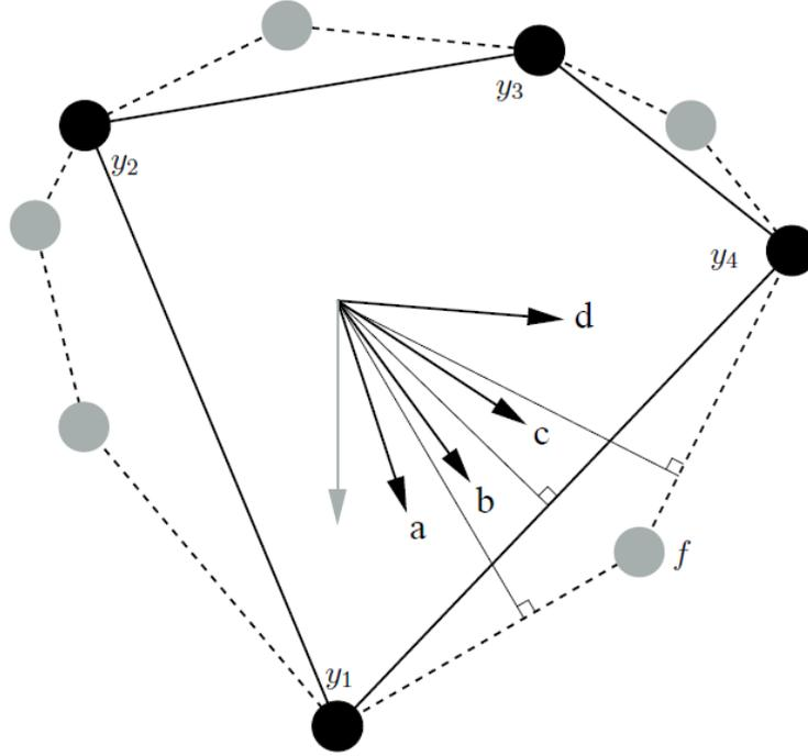
**Figure (22):** A decoding polytope  $\mathcal{P}$  (dotted line) and the convex hull [28]  $P_{ML}$  (solid line) of the codewords  $y_1$  through  $y_4$ . Also shown are the four possible cases (a-d) for the objective function.[14]
