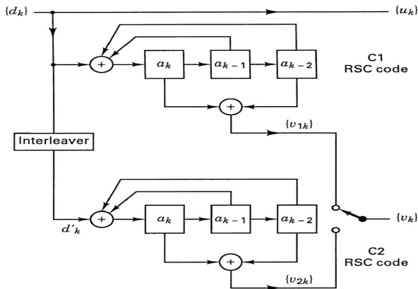
**Figure (18):** Parallel concatenation of two RSC codes.
