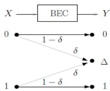
**Figure (3):** The BEC with erasure probability  $\delta$ .
