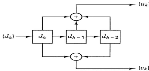
**Figure (16)** : Nonsystematic convolutional (NSC) code.
