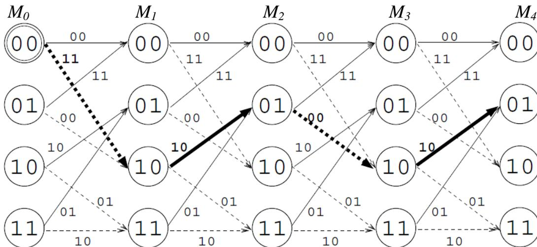
**Figure (24):** A trellis for the rate-1/2 FSM code in figure (23). The trellis has length  $k = 4$ , and five node layers ( $M_0, M_1, M_2, M_3, M_4$ ). As in the state transition table, the bit pairs on the transition edges represent encoded output bits. Each layer of the trellis represents one input bit. The bold path is the path taken by the encoder while encoding the information bits 1010.
