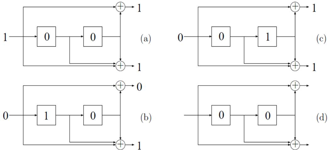
**Figure (25):** The actions of a convolutional encoder for a rate-1/2 convolutional code
