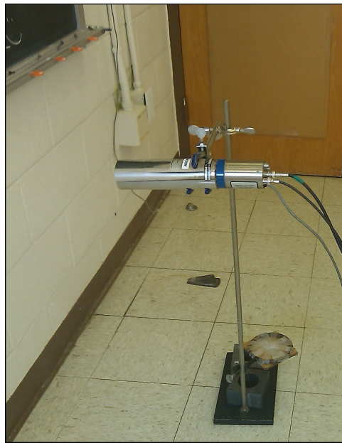
(b) ^{60}\text{Co} source locations. The blackboard is on the y = 0 plane and the wood door is on the x = 0 plane. The detector is at location 6.
