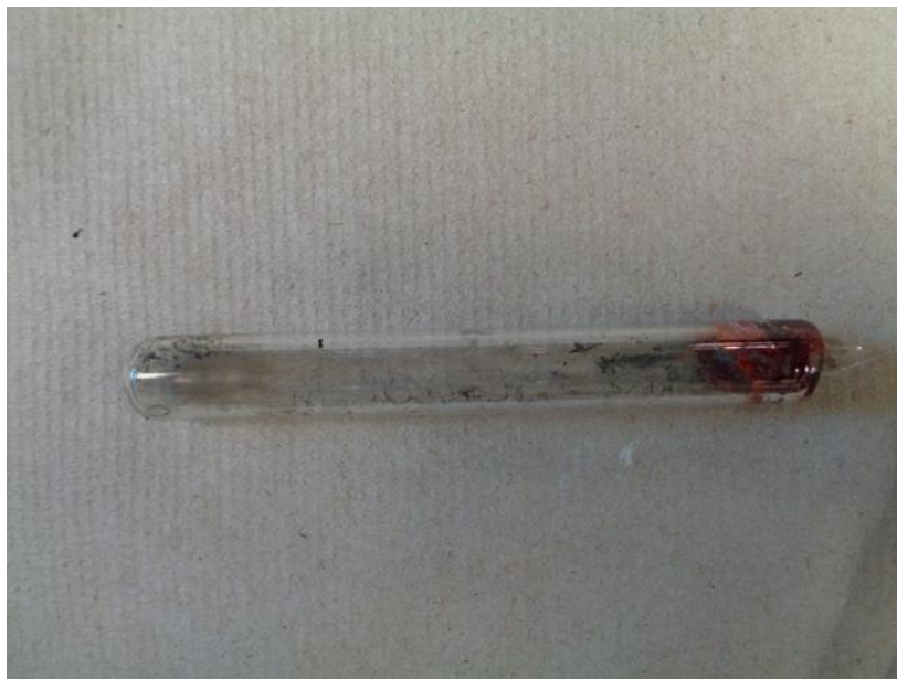
Figure 2.12 Glass tube after growth of bulk black phosphorus
