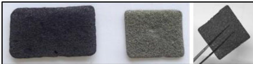
Figure 2.26 | Nickel foam (center), three-dimensional graphene before (left) and after (right) etching the nickel template.
