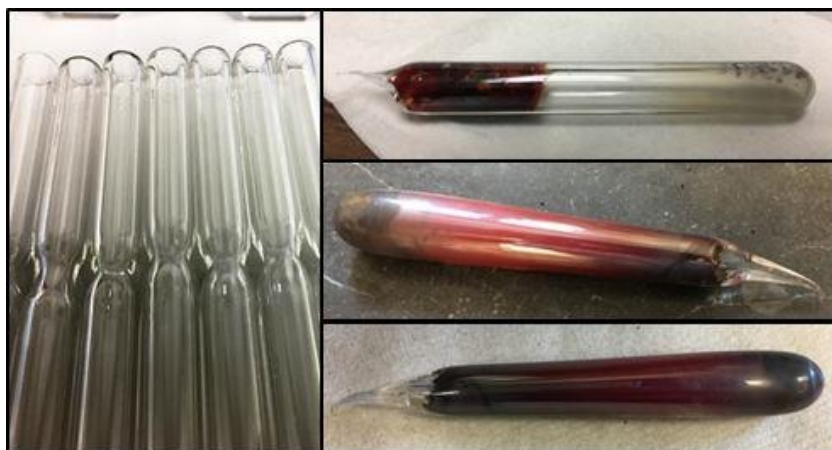
Figure 2.30 | Pyrex tubes before sealing and evacuated glass (Pyrex) tube after annealing at 600 °C.
