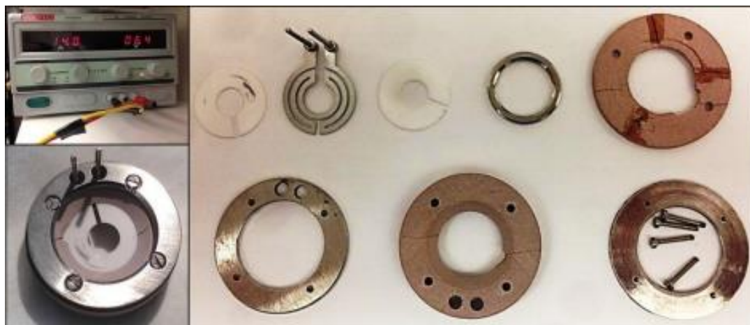
Figure 2.11 | Compact resistive heater (80 W), heater components, and DC power supply.
