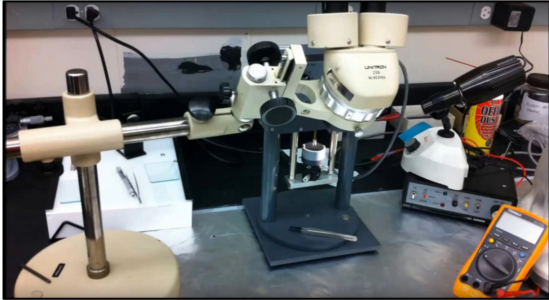
Figure 2.9 | The Micro EDM System and Optical Zoom Microscope.
