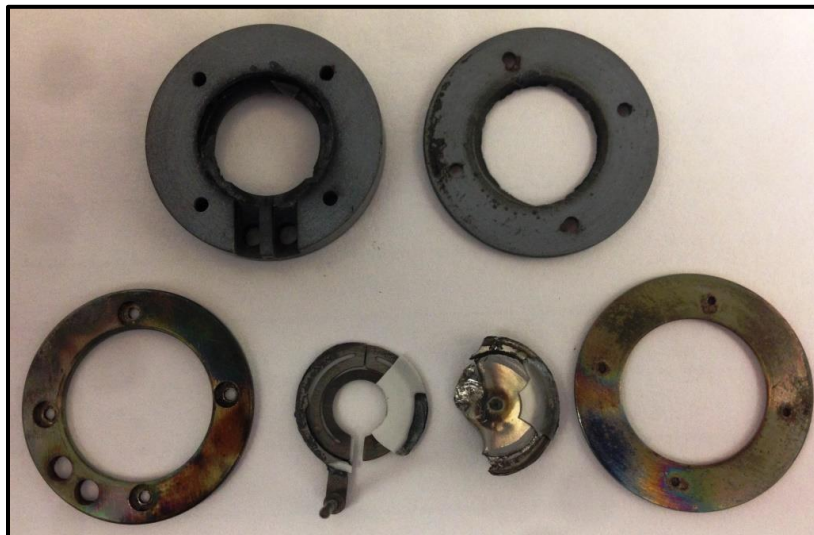
Figure 2.12 | Burned heater components due to excess of current into the metal resistor.
