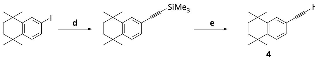
**Scheme 8:** Synthesis of TMNA (4). d) 1.2 eq. TMSA, 1% Pd(PPh<sub>3</sub>)<sub>2</sub>Cl<sub>2</sub>, 1% CuI, Et<sub>3</sub>N; e) 4 eq. Na<sub>2</sub>CO<sub>3</sub>, MeOH/10% H<sub>2</sub>O
