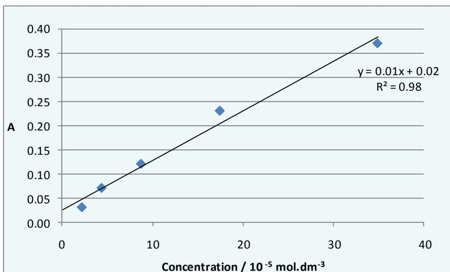
**Figure 17:** Serial Dilution of AT-retinol. Solutions were made up at a range of concentrations from 0.10000 mg/ml to 0.00156 mg/ml. The absorbance (A) of each solution at  $\lambda = 335 \text{ nm}$  was measured and plotted against concentration.  $R^2$  (the coefficient of determination) **Error! Bookmark not defined.** was calculated to be 0.98, showing excellent agreement between concentration and the absorbance measured, confirming pipetting accuracy.
