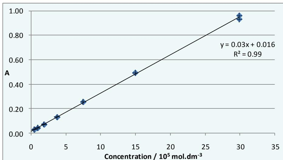
**Figure 16:** Serial dilution of EC23. Solutions were made up at a range of concentrations from 0.10000 mg/ml to 0.00156 mg/ml. The absorbance (A) of each solution at  $\lambda = 306$  nm was measured and plotted against concentration.  $R^2$  (the coefficient of determination)<sup>ix</sup> was calculated to be 0.99, showing excellent agreement between the concentration and the absorbance measured, confirming pipetting accuracy.
