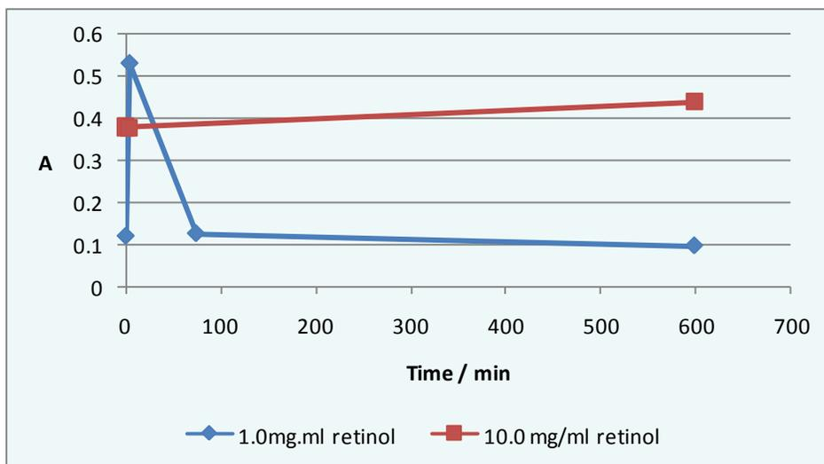
**Figure 19:** AT-Retinol unloading assay. AG1-X2 beads were soaked in AT-retinol in DMSO solution. The excess solution was removed and replaced by fresh DMSO. The absorbance at  $\lambda = 284$  nm of samples was plotted against time to assess the rate at which retinol is released from the beads.
