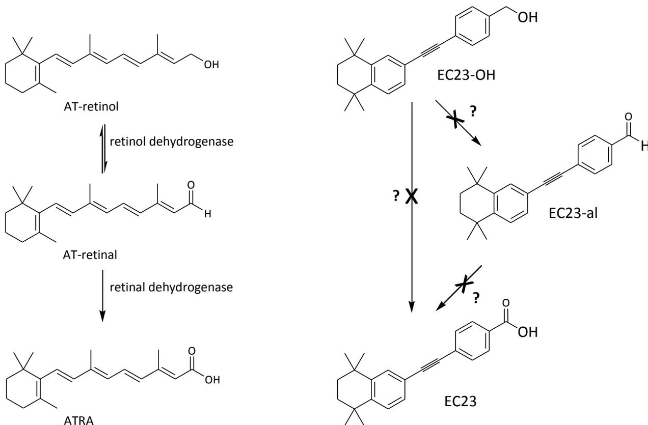
**Scheme 2:** *Left hand side:* A schematic showing the metabolism of AT-retinol to ATRA, via AT-retinal. There is much evidence that this occurs. *Right hand side:* It is currently believed that the body is unable to metabolise synthetic retinoids such as EC23 along the same route as its natural analogue.
