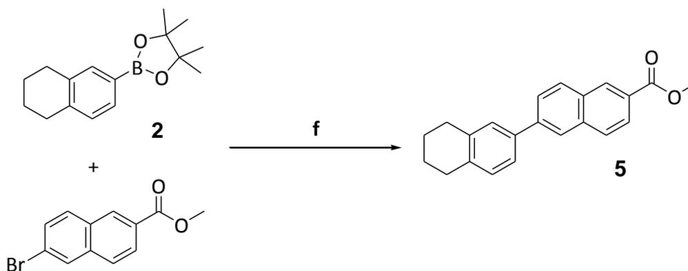
**Scheme 9:** Synthesis of methyl 5',6',7',8'-tetrahydro-2,2'-binaphthyl-6-carboxylate (**5**) f) 2% Pd(dppf)Cl<sub>2</sub>, 2 eq. K<sub>3</sub>PO<sub>4</sub>, 5:1<sup>i</sup>PrOH/H<sub>2</sub>O, 80°C
