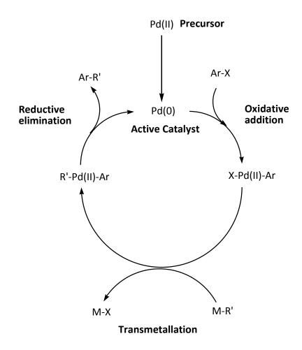
**Scheme 3**: Generic catalytic cycle for palladium-catalysed cross-coupling reactions.
