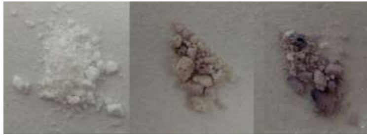
Figure 6.3 Photographs of ninhydrin treated powders after reaction with octanediamine (RHS) and ethanediamine (MIDDLE), compared against untreated polyHIPE powder (LHS)
