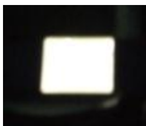
Figure 3.21 – Photograph of white light emitting single layer device based on co-polymer 182. Device architecture: ITO // PEDOT:PSS (50 nm) // 182 (69 nm) // LiF (0.8 nm) // Al (92 nm) operating at 11V
