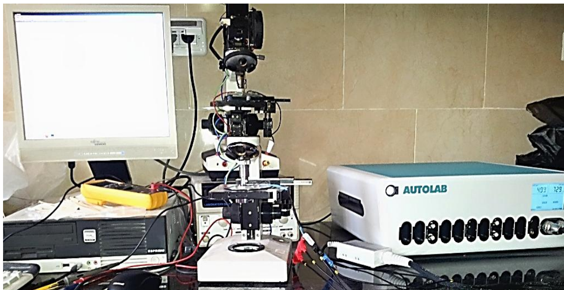
Fig. 3.5 Autolab AUT 85276 Potentiostat- Gelvanostat with frequency response analyzer FRA 32 Module.
