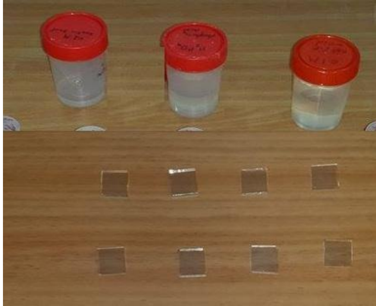
Fig. 4.20 The pre-treatment of the FTO substrates using \text{HCl} , \text{H}_3\text{PO}_4 , and \text{HNO}_3 .
