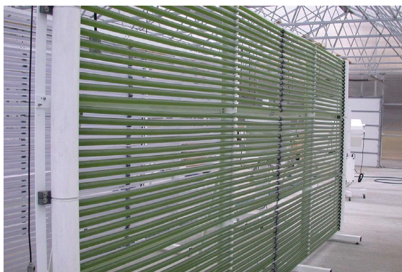
Figure 1.4 Tubular photobioreactor for algae production. Taken from Greenwell et al. 51
