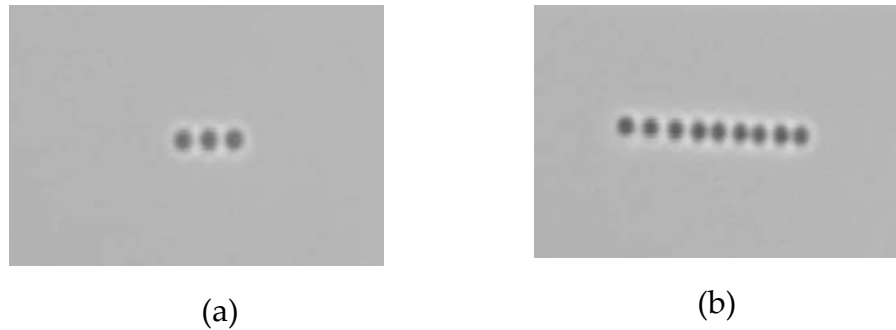
Figure 3.17: Build-up of a line of uncoated 881 nm silica particles showing (a) uniform separations of 3D ; and (b) modulated ‘pairs’.
