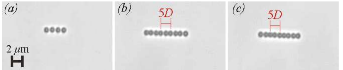
Figure 3.9: Lines of 800 nm PS particles showing (a) uniform spacings of 3D , which subsequently rearranges to (b) pairs, and (c) triplets
