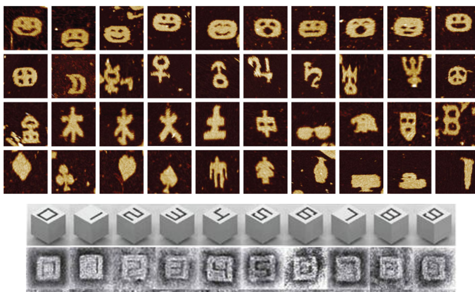
Figure 1.5: The top image shows a series of AFM images of clusters formed from DNA tiles [reproduced from Wei et al. 85 ]. The bottom image shows DNA brick structures with the Arabic digits carved into one face, the top row are representative diagrams where are the bottom contains TEM images of clusters [adapted from Ke et al. 86 ].
