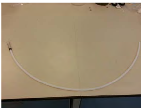
Fig. 2.5 PTFE tubing and plastic syringe used for sampling SVC reactions.
