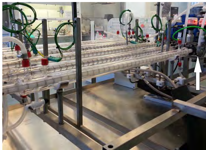
Fig. 2.9 PPU in operation with arrow indicating the position of the pneumatic valve dousing point at the top of the column.
