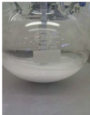
Fig. 2.11 Stirred flask reactor with slurry mixture kept in suspension by stirrer.
