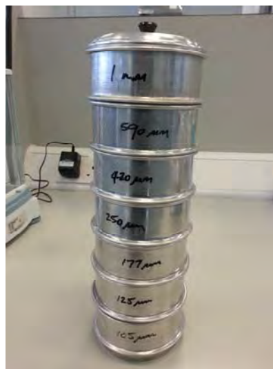
Fig. 2.17 Picture of sieve meshes used for PSD determination, with the largest mesh size of 1 mm at the top and the smallest mesh size of 106 \mu\text{m} at the bottom.
