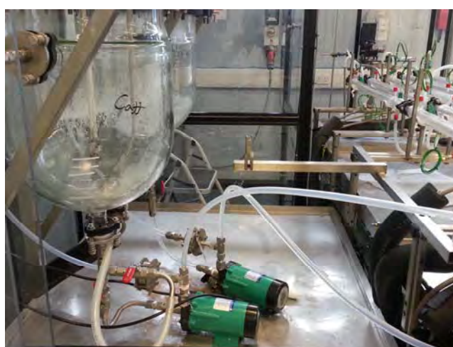
Fig. 2.7 Centrifugal pump used in circulating the API and coformer slurry mixture in PPU set up.
