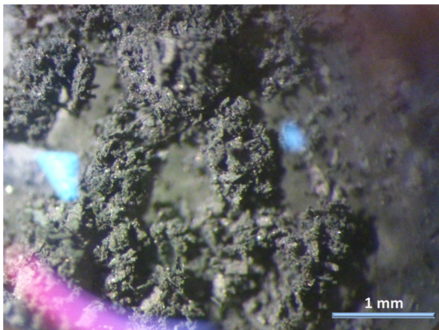
Figure 89: Polycrystalline solid of Cs 2 (C 14 H 10 ) under 40× magnification, the thick blue line represents 1 mm length.
