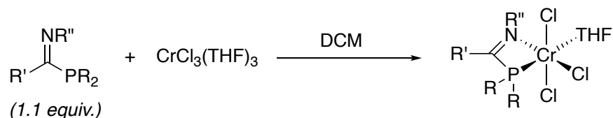
Scheme 2.44: Attempted synthesis route to Cr III -PCN complexes, following modification of the method reported by Labinger and Bercaw et al. 33
