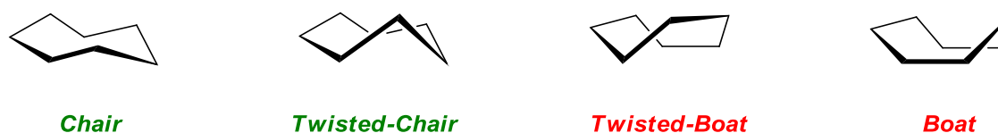
Figure 4.2 Possible conformations of cycloheptane and other 7-membered rings. Chair and twisted-chair conformers are of lower energy than the boat and twisted-boat conformers.
