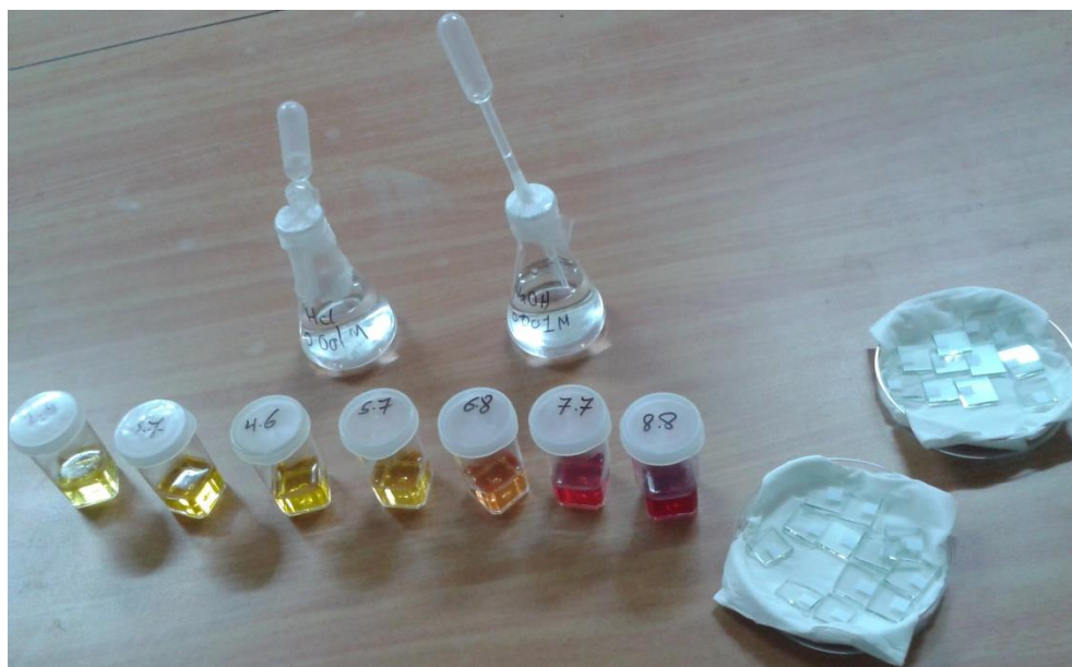
Figure (4.15): Changing the pH of the Haematoxylin dye solutions using hydrochloric acid and sodium hydroxide.
