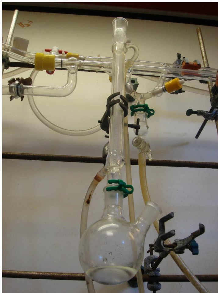
Figure 3.4: The experimental set-up for the synthesis of NaOD.
