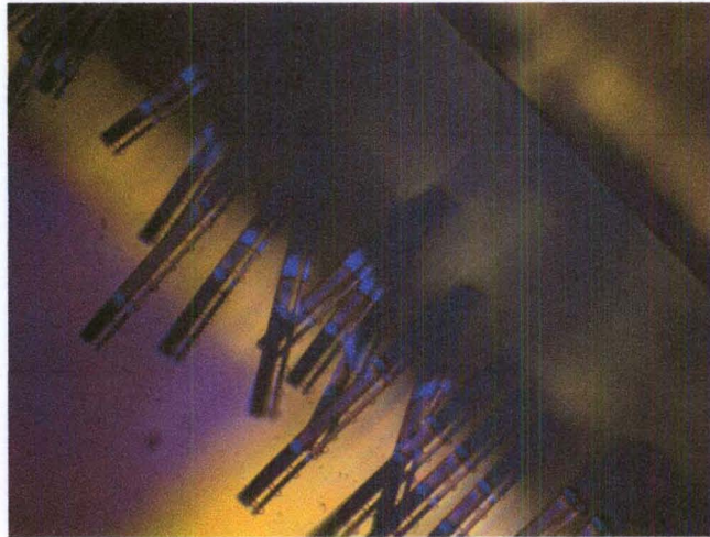
FIGURE 3: Microscopic image of the damaged electrodes after the water flow.
