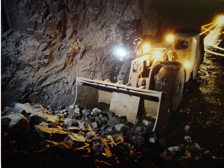
Figure 9.7: Cat R2900 load-haul-dump vehicle working underground.
