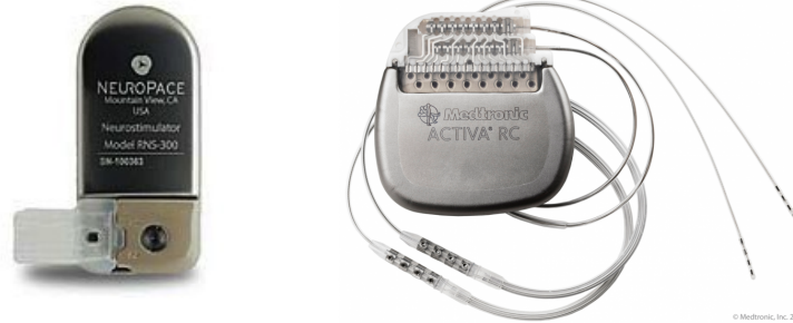
(a) An epileptic seizure control device by NeuroPace Inc., Mountain View, California. (Credit: NeuroPace Inc.)
