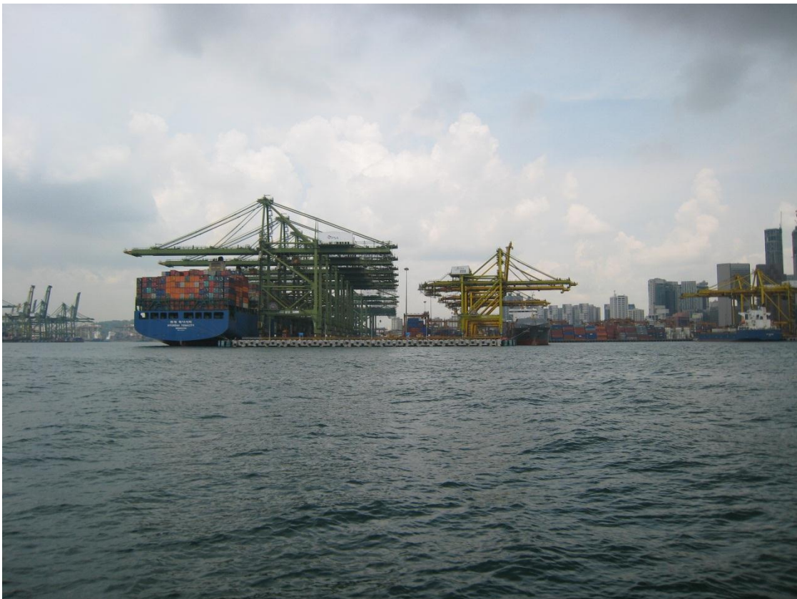
Figure 17 : Example of parallel loading/unloading process between vessel ( left ) and Feeder ( right side ) at the same berth ( own picture in the port of Singapore )
