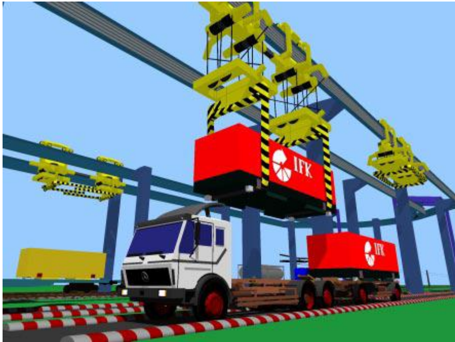
Figure 58 : Handling with electric monorail Concar with parallel movement of truck or train and the hanging multiple lift.( after D.Arnold )
