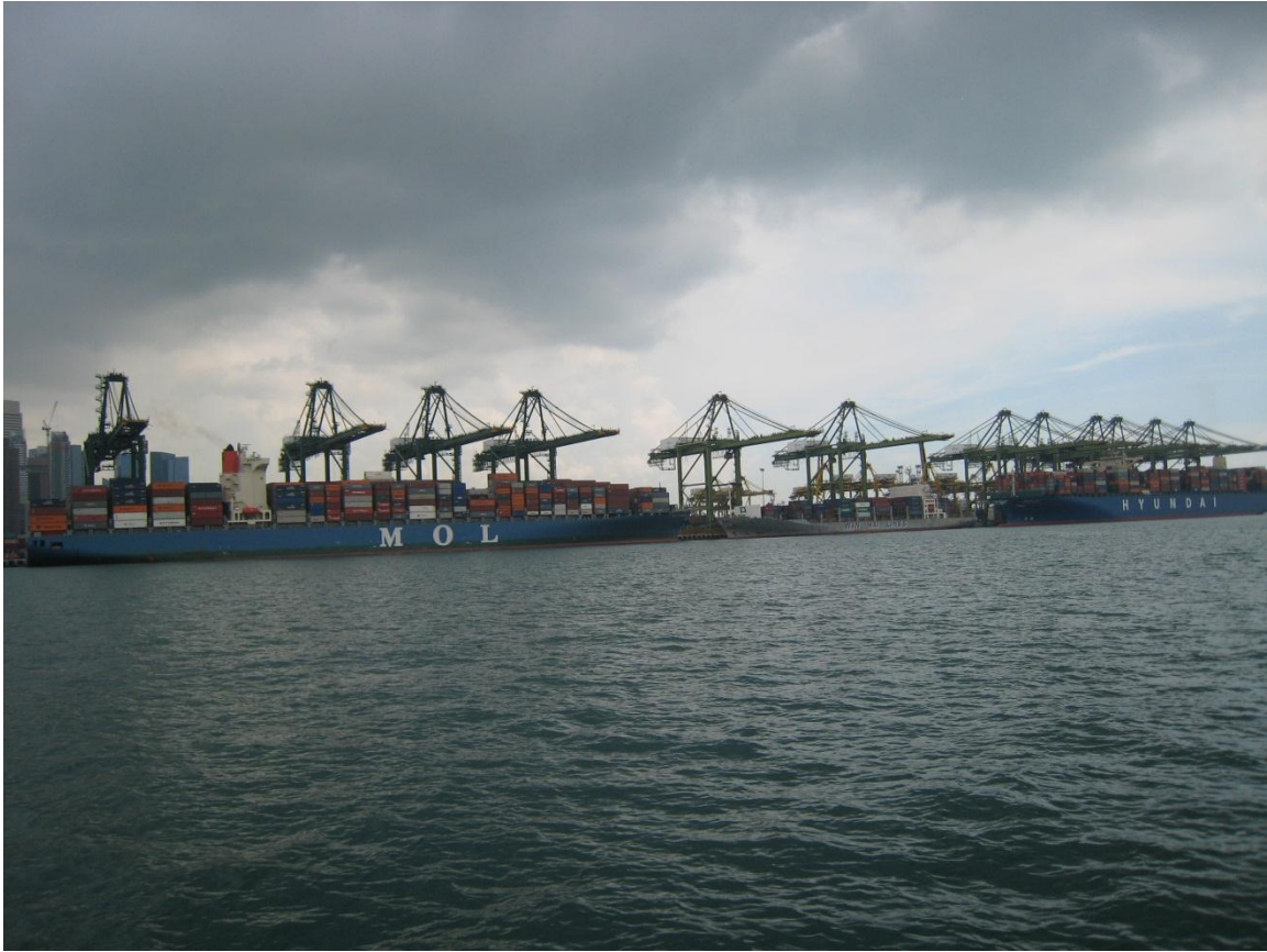
Figure 18 : Example of loading/unloading process of a feeder (middle ) serving 2 vessels at the same berth side. Containers are moved along the berth ( own foto in the port of Singapore )
