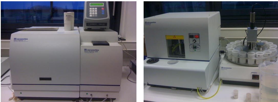
Figure 8: Laser fraction measurement (left) and X-ray sedimentation measurement 5
