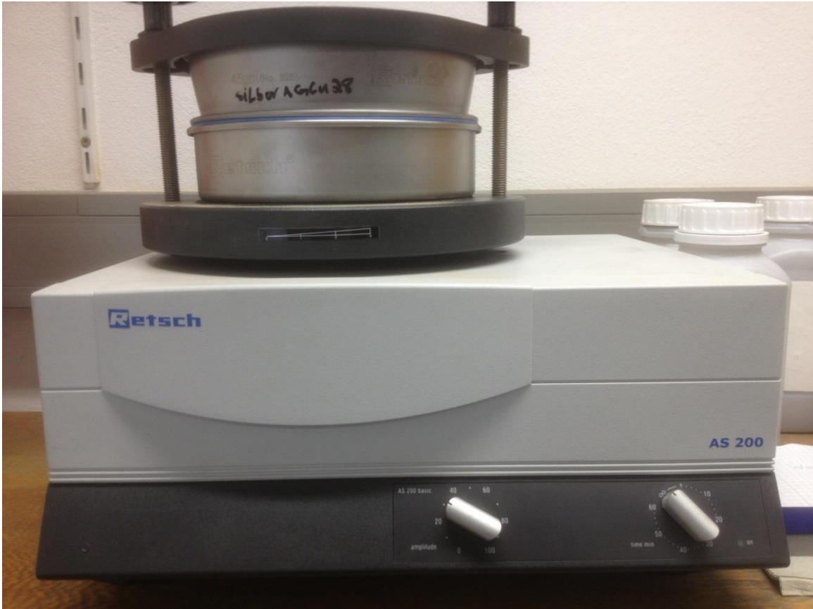
Figure 104: Vibratory sieve shaker with 45 \mu\text{m} test sieve
