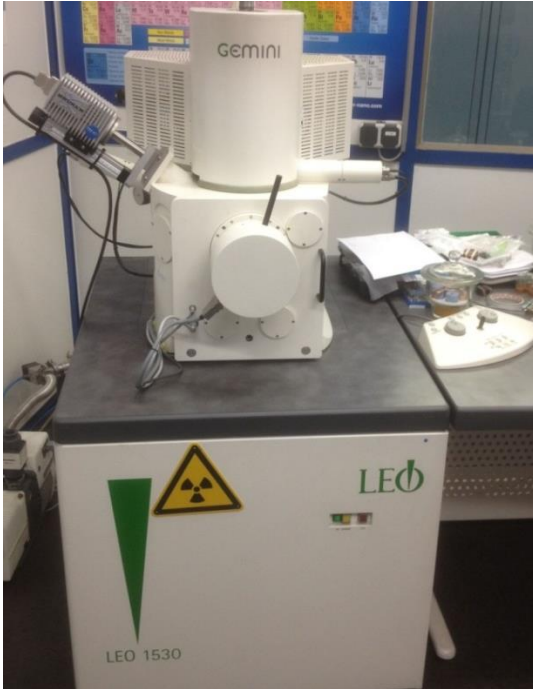
Figure 22: SEM and EDX analyzer Gemini LEO 1530
