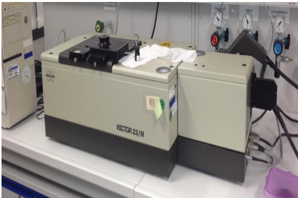
Figure 19: Ulbricht ball and Michelson interferometer
