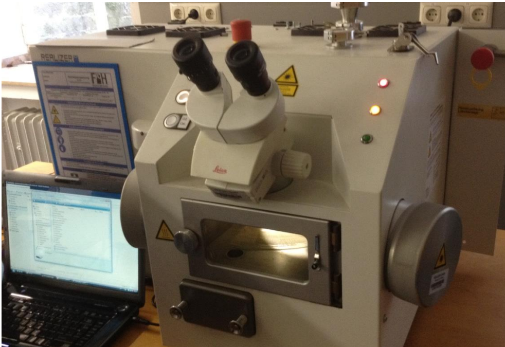
Figure 5: Realizer SLM 50 desktop machine
