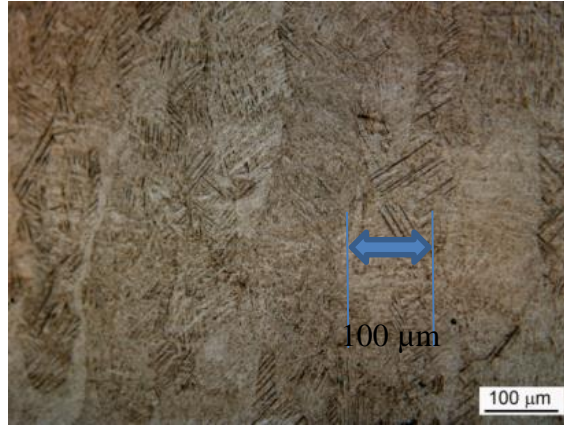
Figure 32 Optical microscopy image of microstructure showing grain boundaries along the melt pool boundary.
