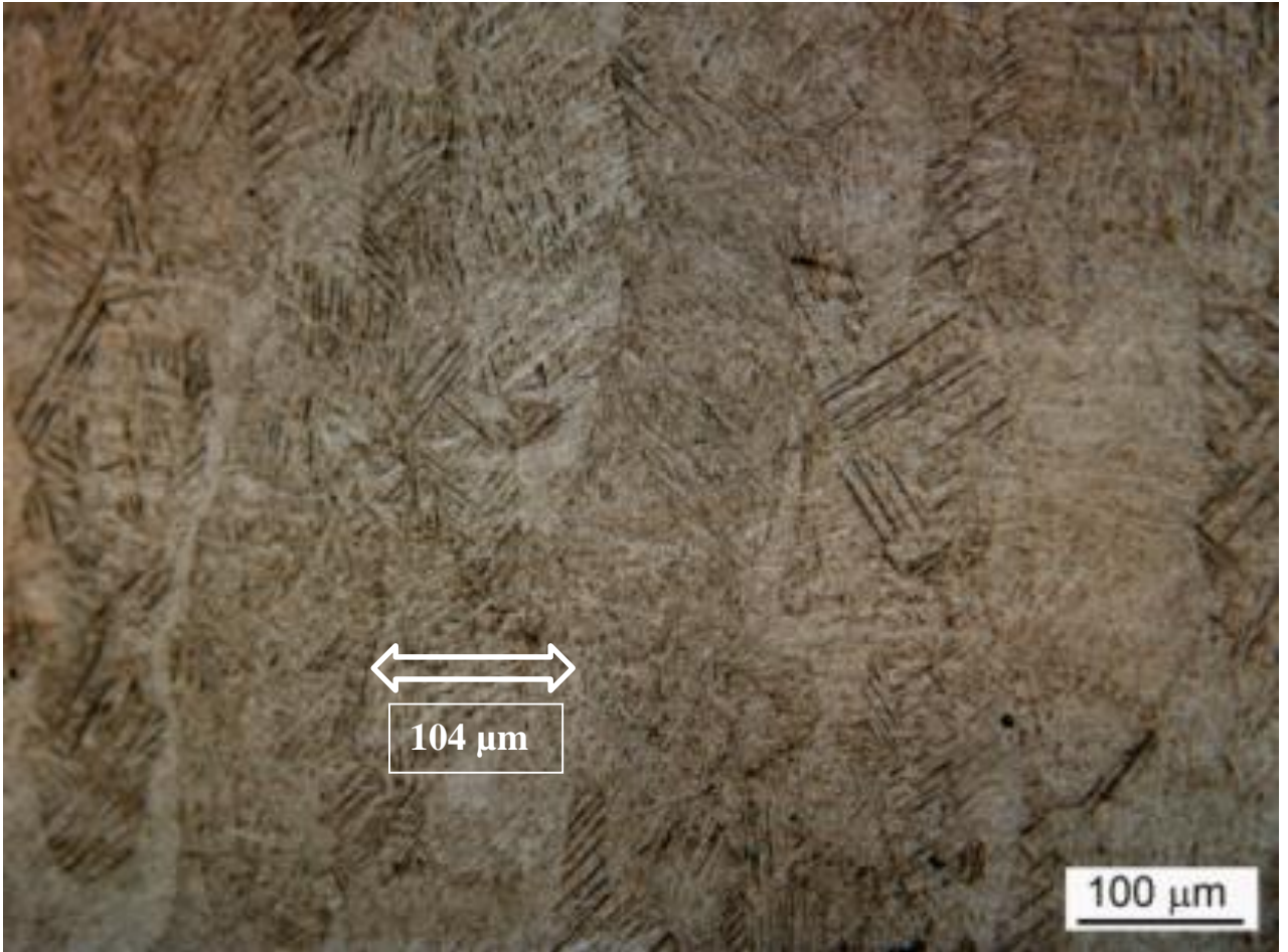
Figure A.14: Transverse prior \beta grain diameter ( \sim 100 \mu\text{m} ).
