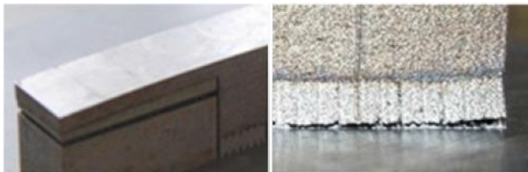
Figure 13 Distortion and delamination in SLM processing [60]
