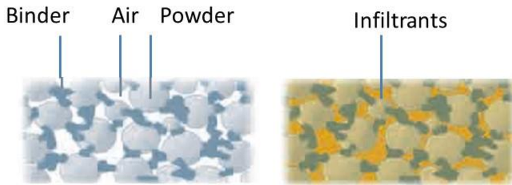
Figure 47: Application of infiltrants (adapted from Z Corporation, 2012b, pp. 10)
