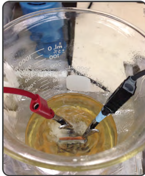
FIGURE 7 - Top view of Stir Design 0 showing anodic sample and cathode support submerged in solution.
