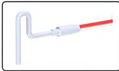
FIGURE 16 - Rendering of the thermocouple implemented in Flow Design 2. The custom made thermocouple features a stainless steel construction, a chemically resistant coating, and a bent neck that reaches above the top of the polishing chamber in order to maintain a low profile.
