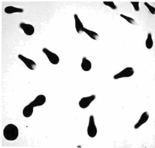
Figure 3.5: Tracks Formation on CR-39 Detectors After Chemical Etching
