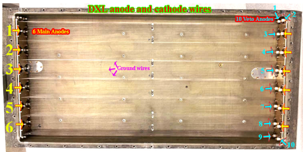
Figure 3.6: DXL anode and cathode wire arrangements
