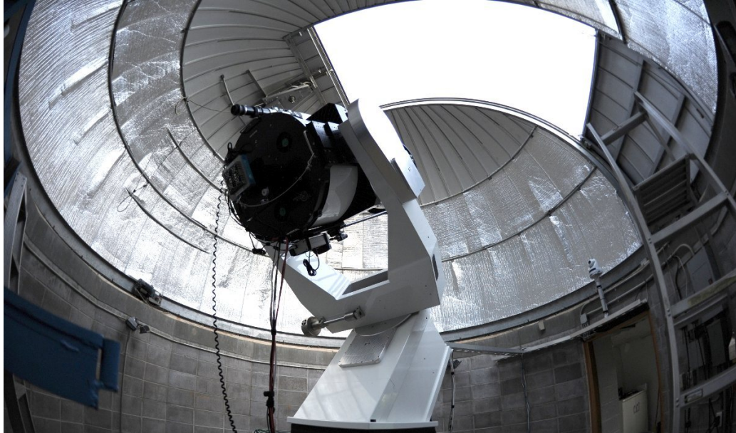
Figure 15. Inside view of MORC telescope enclosure. The inside view shows the upper shutter raised giving access to target altitudes ranging from 38^{\circ} to 90^{\circ} above the horizon.
