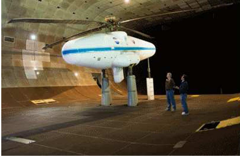
Figure 4.1 UH-60A rotor system installed on the Large Rotor Test Apparatus in the NFAC 40-by 80-foot wind tunnel [23]
